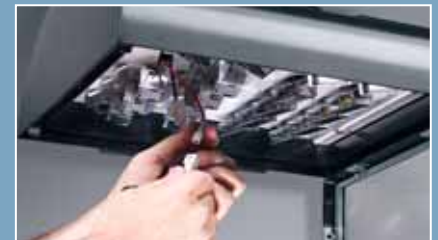
QUICK CONNECT WIRING Install the new MicroEmitter by reconnecting the electrical quick connectors and replacing the mounting screw.
