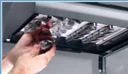
DISCONNECTING THE WIRING Once the MicroEmitter module is released, slowly pull the wiring through the mounting slot to access the electrical quick connectors.
