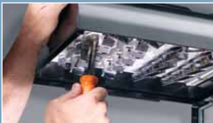
MICROEMITTER MODULE REMOVAL A single removable mounting screw holds MicroEmitter module in place.
